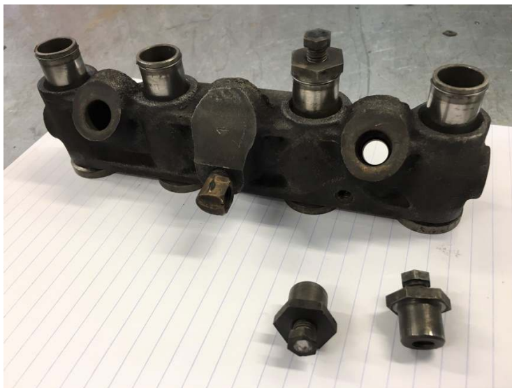
LEFT: THE PHOTO SHOWS FOUR CAM FOLLOWERS IN A BLOCK WITH ONE OF THE SOLID LIFTERS IN PLACE AND TWO AT THE FRONT OF THE PHOTO SHOWING THE ADJUSTING NUT.
